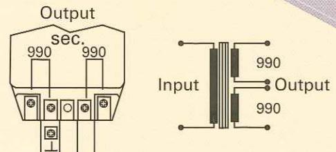
The Low Voltage double output model (striking voltage: <1000V; working voltage: <500V) is highly appreciated by architects and designers for indoor lighting projects, for false ceilings, panels and embedded lightings in general.
